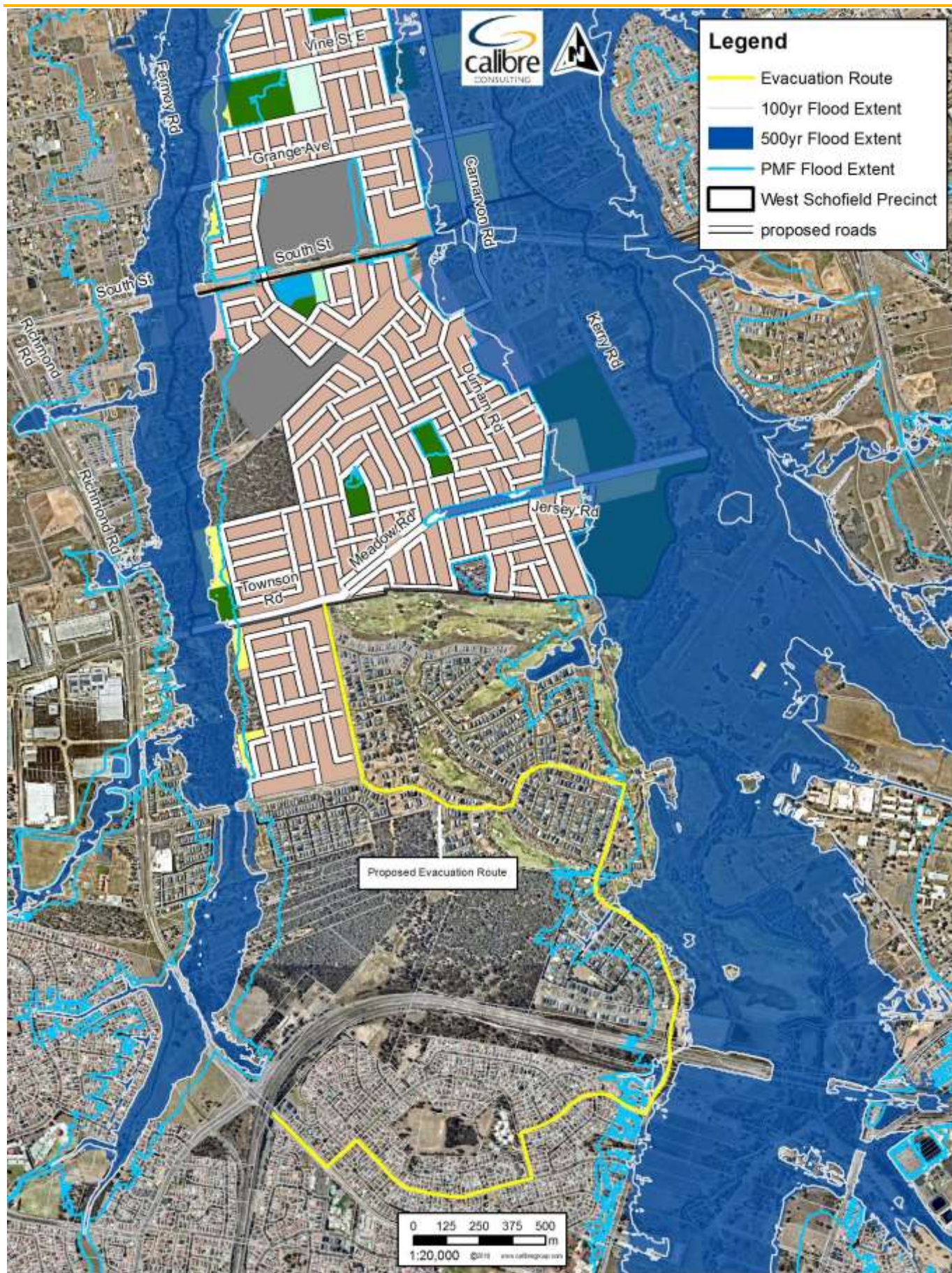
Figure 5.9: Flood Evacuation Route Map
